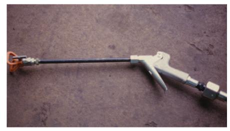
Airless spray wands are available in two general types, a pole gun or a trigger spray wand.
