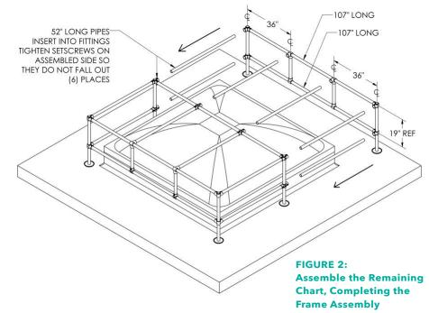
**3.** Assemble remaining parts shown in Fig. 2 tighten all setscrews and torque to 29 lb-ft. **CAUTION: Extreme care should be taken when installing 52" pipes, do not drop them on the skylight dome. Tighten setscrews for 52" pipes on pre-assembled side of frame so they do not fall out.**
