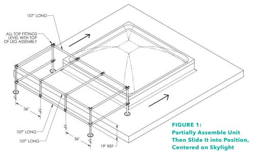
1. Partially assemble skylight frame as shown in Fig. 1 tighten all setscrews and torque to 29 lb-ft.
