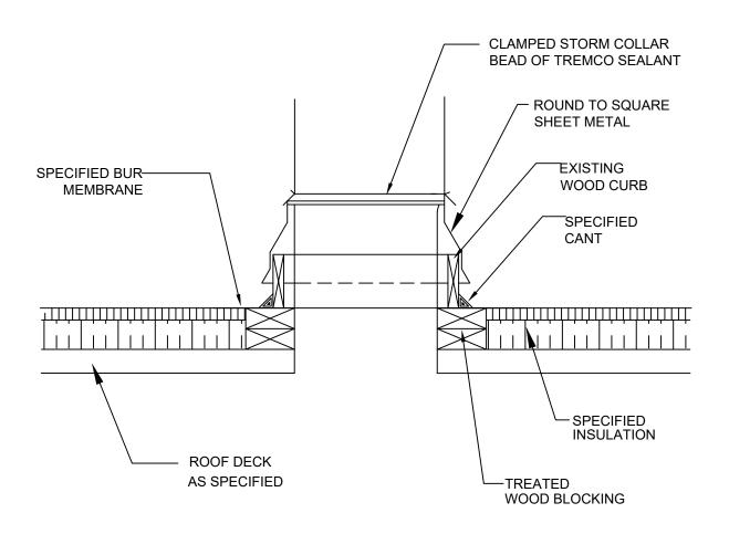
FABRICATED ROUND TO SQUARE SHEET METAL TWO PIECE SOLDERED IN FIELD.
