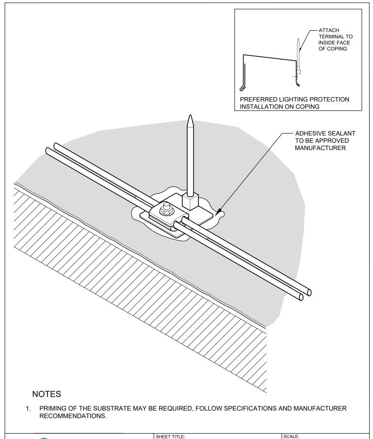
TREMCO Roofing & Building Maintenance SHEET TITLE: LIGHTNING PROTECTION TERMINAL PARTIALLY REINFORCED **RESTORATION**
