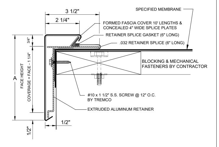
Note: WHEN USED FASCIA CAN BE USED WITH BUR/MB/SINGLE PLY SYSTEMS
