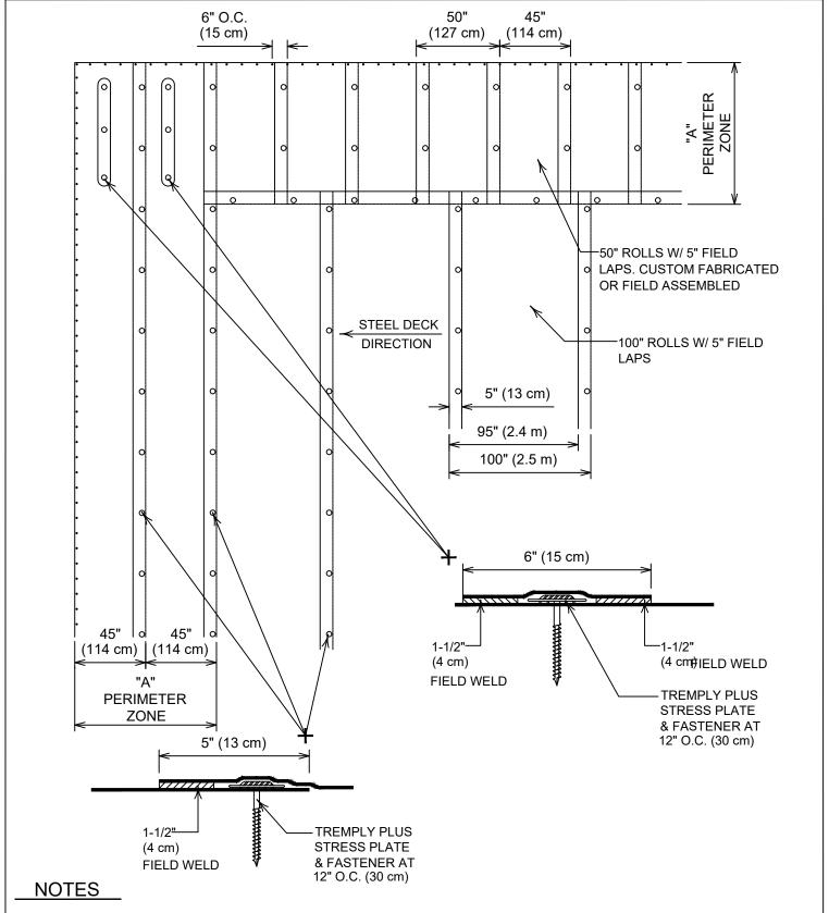
DIMENSION "A" EQUALS 10% OF ROOF WIDTH OR 40% OF BUILDING HEIGHT; WHICH EVER IS LESS, WITH A MINIMUM OF 4 FT. (1.2 M)
