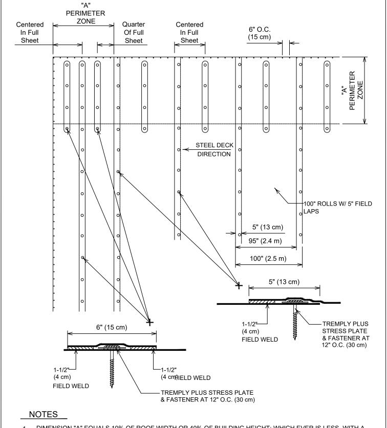
1. DIMENSION "A" EQUALS 10% OF ROOF WIDTH OR 40% OF BUILDING HEIGHT; WHICH EVER IS LESS, WITH A MINIMUM OF 4 FT. (1.2 M)
