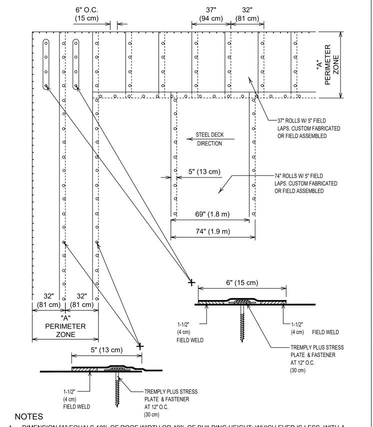
DIMENSION "A" EQUALS 10% OF ROOF WIDTH OR 40% OF BUILDING HEIGHT; WHICH EVER IS LESS, WITH A MINIMUM OF 4 FT. (1.2 M)
