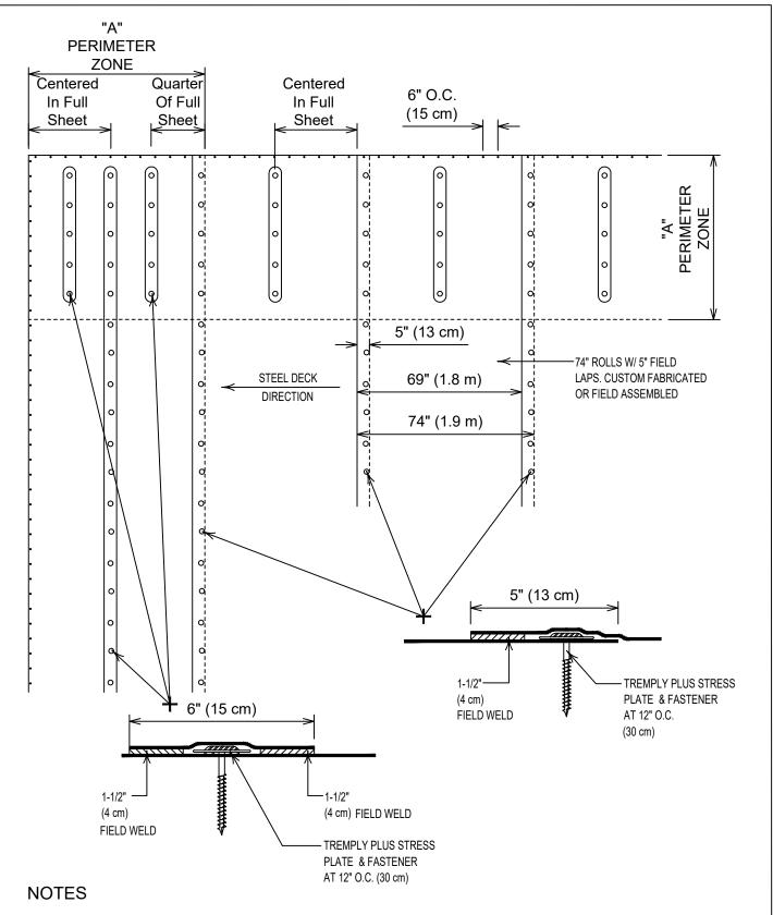
1. DIMENSION "A" EQUALS 10% OF ROOF WIDTH OR 40% OF BUILDING HEIGHT; WHICH EVER IS LESS, WITH A MINIMUM OF 4 FT. (1.2 M)
