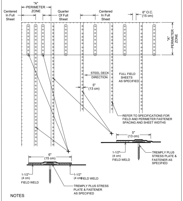
DIMENSION "A" EQUALS 10% OF ROOF WIDTH OR 40% OF BUILDING HEIGHT; WHICH EVER IS LESS, WITH A 1. MINIMUM OF 4 FT. (1.2 M)
