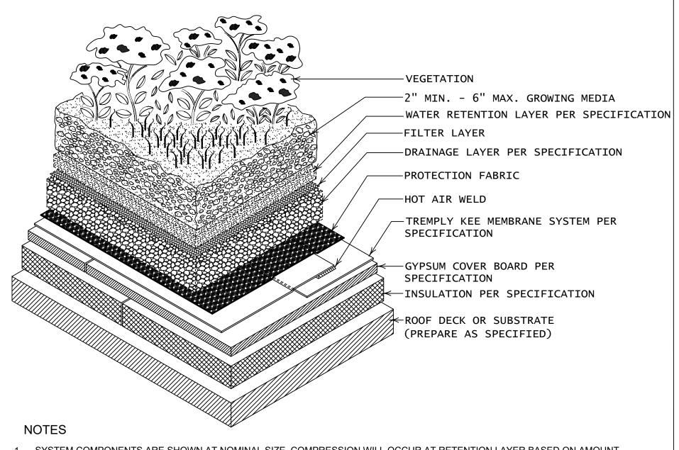
1. SYSTEM COMPONENTS ARE SHOWN AT NOMINAL SIZE, COMPRESSION WILL OCCUR AT RETENTION LAYER BASED ON AMOUNT (HEIGHT/VOLUME) OF GROWING MEDIA PLACED ON SYSTEM. MAXIMUM COMPRESSION 1/4"
