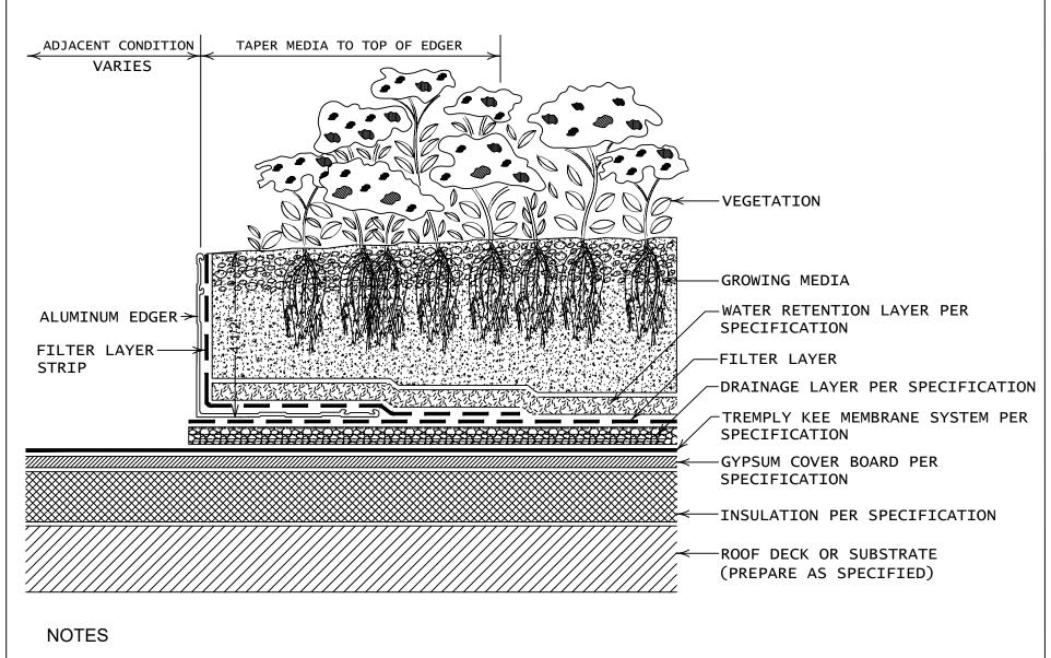
1. SYSTEM COMPONENTS ARE SHOWN AT NOMINAL SIZE, COMPRESSION WILL OCCUR AT RETENTION LAYER BASED ON AMOUNT (HEIGHT/ VOLUME)
