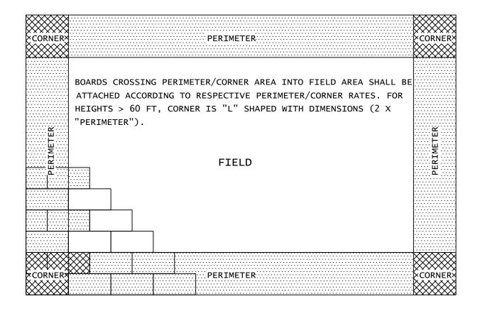
PERIMETER AND CORNER WIDTH DIMENSIONS ARE DETERMINED BASED ON THE LESSER PRODUCT DERIVED BY MULTIPLYING THE BUILDING HEIGHT BY .4 (40%) OR THE LESSER BUILDING DIMENSION BY .1 (10%).
