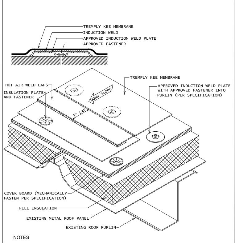
1. REFER TO DETAIL IWS1 FOR PROPER PLATE SECUREMENT TO ENSURE MAXIMUM MEMBRANE TO PLATE BONDING. WHEN INSTALLING MULTIPLE LAYERS OF INSULATION ALL END JOINTS SHALL BE STAGGERED.
