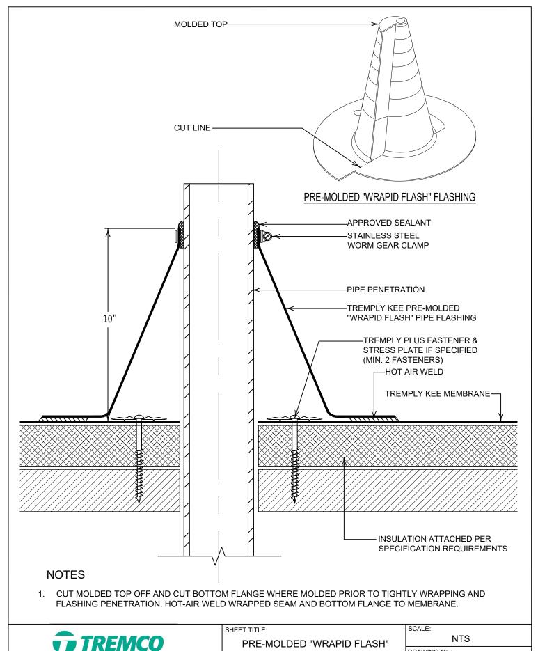
PIPE PENETRATION FLASHING
