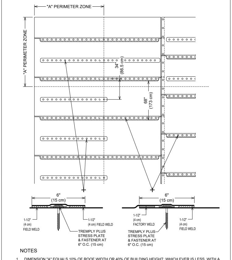
1. DIMENSION "A" EQUALS 10% OF ROOF WIDTH OR 40% OF BUILDING HEIGHT; WHICH EVER IS LESS, WITH A MINIMUM OF 6 FT. (1.2 M)
