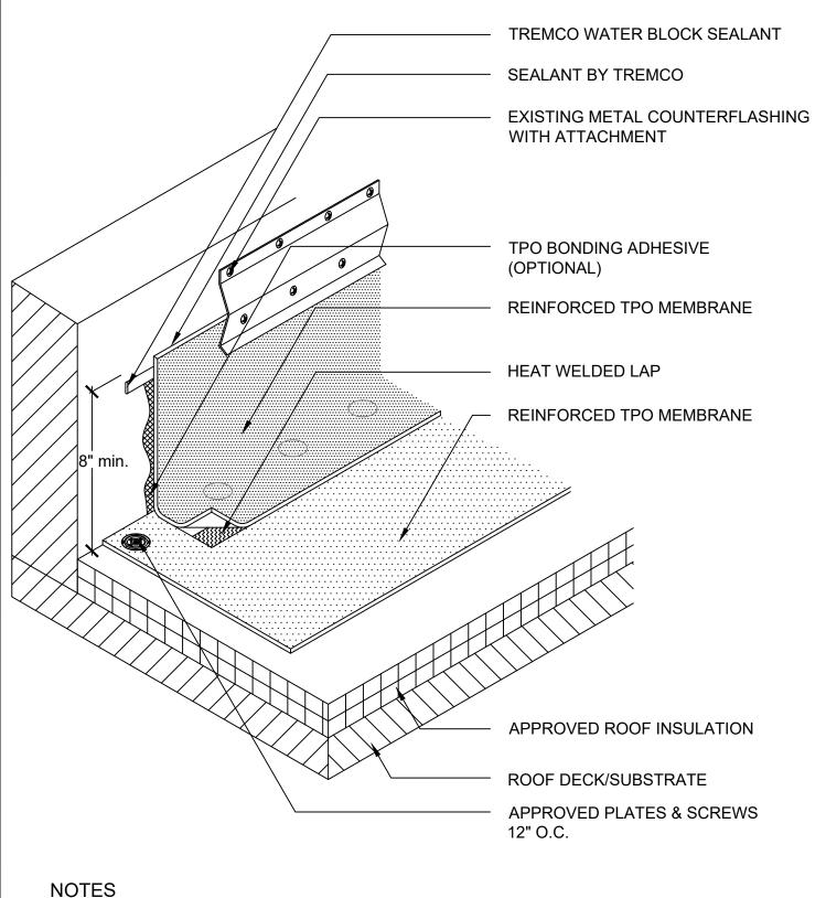
1. APPLY TPO AND PVC CUT EDGE SEALANT TO ALL CUT REINFORCED TPO AND PVC EDGES.
