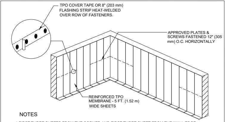
1.FIRST THREE SHEETS FROM THE CORNER AND FIRST THREE SHEET FROM THE WALL EDGE REQUIRE A ROW APPROVED PLATES AND FASTENERS 12" O.C. MID WAY UP THE WALL AS SHOWN.
