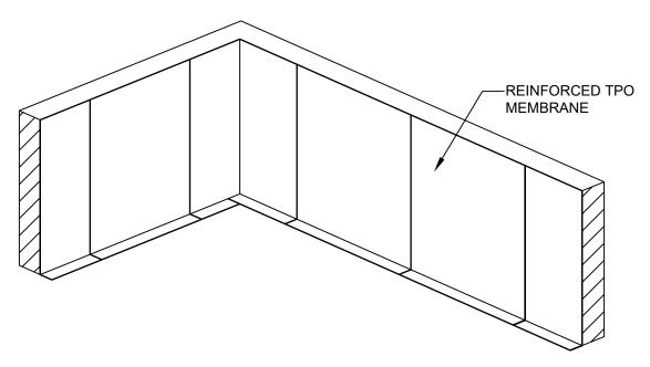
1. FIRST SHEET FROM THE CORNER AND FIRST SHEET FROM THE WALL EDGE ARE 10' (3.05 m) WIDE. ALL SHEETS IN BETWEEN ARE 20' (6.10 m) WIDE.
