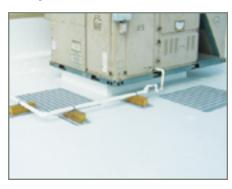
These walkpads are designed for use with Tremco Roofing TPA systems to provide protection around rooftop equipment. They are a polyester reinforced, thermo-plastic membrane engineered to provide a defined, slip-resistant, trafficbearing walking surface. The low profile TPA walkpad is mold, mildew and chemical resistant and is easy to clean.
